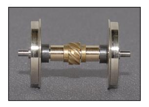
As with all of Ultrascale's replacement wheelsets, (I use specifically nickelsilver), I've always found they maintain 100 % of the loco's traction, whilst improving the pick up qualities by at least 50 % and wheel clarity by 100 %!.
